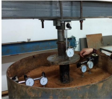
Figure 8. Stone column model test in laboratory scale
