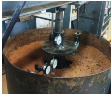
Figure 11. Stone column model test after static loading
