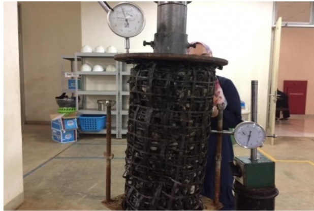
Figure 4. Artificial column compressive strength test
